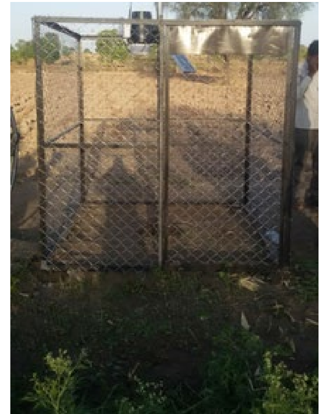
Figure 3 Automated Weather Stations for Hyper-locale crop advisories
